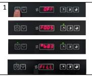
With the hood closed: Press and hold the on/off button for a few seconds. The **L1** light will turn **green** and the display shows the scrolling software version uploaded on the machine.
