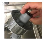
Every 20 or 30 cycles, inspect the removable filter inside the machine for food debris and empty and clean as required. IMPORTANT - Do not operate the machine whilst this filter is
