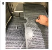
Every 20 or 30 cycles, inspect the top filters inside the machine for food debris, if heavily soiled perform a **P0** program and then remove carefully and clean as required.
