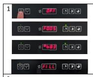
**With the door closed**: Press and hold the on/off button for a few seconds. The **L1** light will turn **green** and the display shows the scrolling software version uploaded on the machine.
