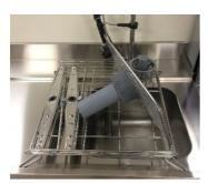
Lift the hood and remove the basket guide, all the filters and the upper and lower wash and rinse arms. Clean and inspect the wash and rinse arm nozzles and wash arm hubs for blockages and ensure the filters are free from any dirt or grime
