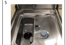
With the machine now empty, with a warm damp cloth wipe all the grey plastic parts, as well as around the door gullies and anywhere else dirt and grime is visible inside and around the machine
