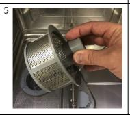
Every 20 or 30 cycles, inspect the removable filter inside the machine for food debris and empty and clean as required. IMPORTANT - Do not operate the machine whilst this filter is removed
