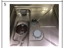
With the machine now empty, with a warm damp cloth wipe all the grey plastic parts, as well as around the door gullies and anywhere else dirt and grime is visible inside and around the machine
