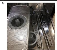
Open the door and remove the all the filters and the upper and lower wash and rinse arms. Clean and inspect the wash and rinse arm nozzles and wash arm hubs for blockages and ensure the filters are free from any dirt or grime
